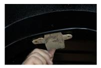
**bracket hanging down in the photo.** The upper coil over mount bar brackets differ from side to side. The right side (passenger) has an extra side plate attached to it. Place both upper coil over mount brackets into position as shown below.
