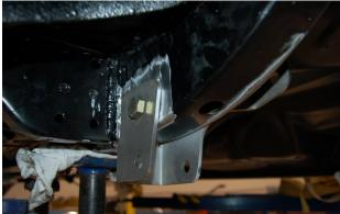
The pictures to the left show the forward frame bracket on the inside and outside of the rail, firmly against the sheet metal lip.
