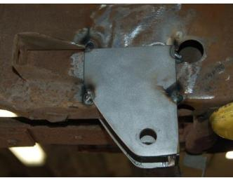
The picture to the right is the inside of the rail. The bracket sits squarely against the parking brake cable clip. The picture to the left shows the bracket on the outside of the rail, firmly against the sheet metal lip.
