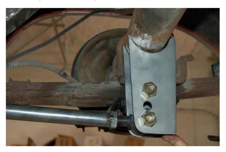
9. When you are satisfied that the bracket is in the appropriate location, place a tack weld in the corners of the bracket just to hold it into position. If you need to make an adjustment later you will only have to cut through a few tack welds.
