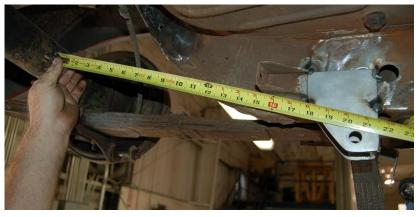
5.Measure the distance from the forward frame bracket mounting hole to the forward face of the differential as shown in the picture below. It should measure 20.500". Measure both sides to make certain the differential is square.
