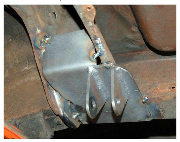
13. You are now ready to attach the upper trailing arms to the upper trailing mounting bar. Just hand tighten the bolts. Attach the upper trailing arm differential tabs to the differential end of the upper trailing arm. Each side gets one long tab and one
