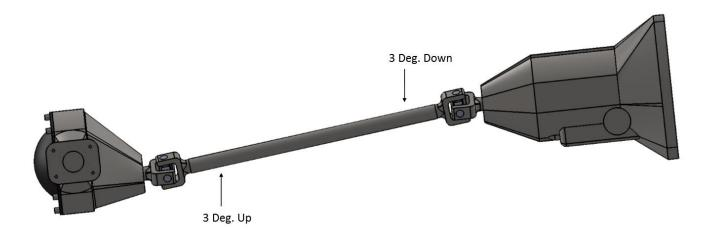
7. Once you have the pinion angle set and the differential properly centered side-to-side, place the brackets that are attached to the lower trailing arms onto the differential. When you are satisfied that the brackets are in the appropriate location and perpendicular to the differential axle tubes and the ground, place a tack weld in the corners of the brackets just to hold them into position. If you need to make an adjustment later you will only have to cut through a few tack welds.
