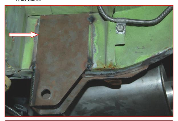
The picture above shows the forward frame bracket on the outside of the rail, firmly against the sheet metal lip (arrow). Do this on both sides then measure each bracket distance from a fixed point on each side of the chassis. Make fine adjustments to ensure they are positioned at equal distances and square.
