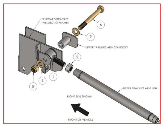
3. Prepare both upper and lower trailing arms and screw the rod ends in until about three threads are showing between the jam nut and the body of the rod end. Only hand tighten the jam nut. The length of both upper trailing arms should match each other as should the lower trailing arms.
