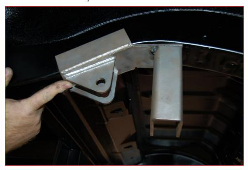
5. Install the left side (driver) upper coil-over mount bracket onto the left chassis rail as shown below. Use the other bump stop screw from Step 3. Installation is pictured below. Tack weld into place.
