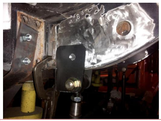
The picture above shows the forward frame bracket on the outside of the rail, firmly against the sheet metal lip. Do this on both sides then measure each brackets distance from a fixed point on each side of the chassis. Make fine adjustments to ensure they are positioned at equal distances and square.
