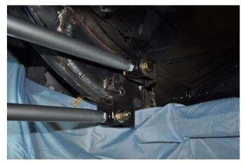
The picture above shows the forward frame bracket on the outside of the rail, firmly against the sheet metal lip. Do this on both sides then measure each brackets distance from a fixed point on each side of the chassis. Make fine adjustments to ensure they are positioned at equal distances and square.
