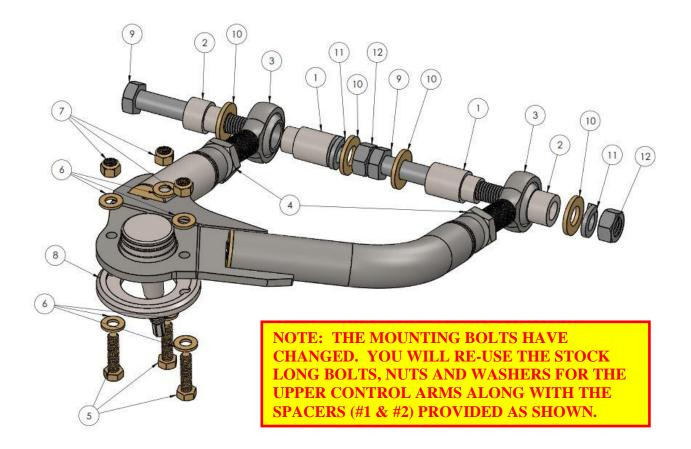
11. Using anti-seize on the threads, install the rod ends and jam nuts into the machined ends of the upper control arms, being careful not to cross-thread. You
