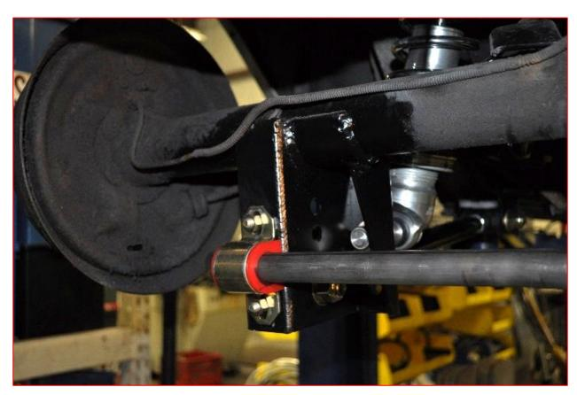
5. Place the sway bar into position on the rear trailing arm brackets and install the steel brackets over the red bushings and into the two lowest holes on the trailing arm brackets.
