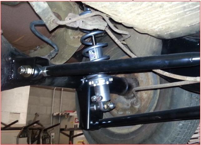
below the height adjustment. Turn the valve all the way counterclockwise and then count ten turns clockwise. This will provide a preliminary setting for the coil over adjustments.
