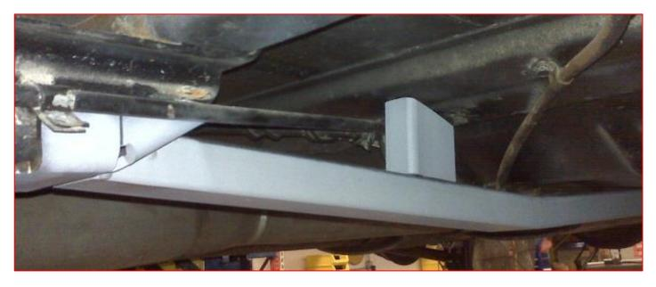
7. When the long bars have been tack welded into position, insert the small wedge-
