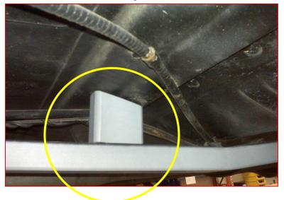
shaped bars as shown in the picture below. Make certain they meet the stamped bracket on the underside of the vehicle. Depending on the condition of your floor pans, some of the wedge-shaped part will need to be trimmed. Do not force it into position. Trim it so it slides in easily as it will be welded into position on the sub-frame connector and the floor brace. Tack weld into position.
